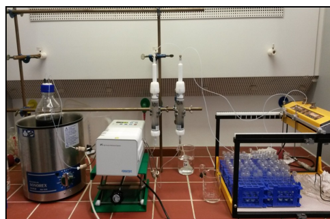
(Above) Column setup for nanoparticle transport experiment (Source: University of Vienna). (Right) Heads of monitoring arrays for in-situ susceptibility measurement (© VEGAS/University of Stuttgart, Germany)
