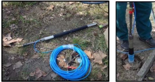
Photos 2a and 2b. The injection rod being inserted. Source: Judith Nathanail.
