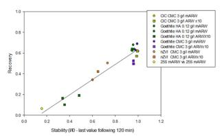
Figure 3. Particles recovery vs. stability laboratory experiment results.
