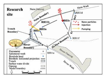
Figure 2.The injection site and proposed injection boreholes. The pumping borehole, as well as the pumping station downgradient, will minimise potential particle loss to the wider groundwater environment (taken from Kurtzman *et al.*, 2005).
