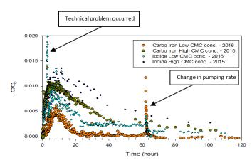
Figure 5. Breakthrough curve of Carbo-Iron® and iodide in both field experiments at RH11A.
