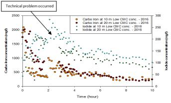
Figure 6. Carbo-Iron® and iodide concentrations at RH11C.
