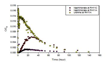
Figure 4. Uranine and Naphthionate recoveries during the preliminary tracer tests.
