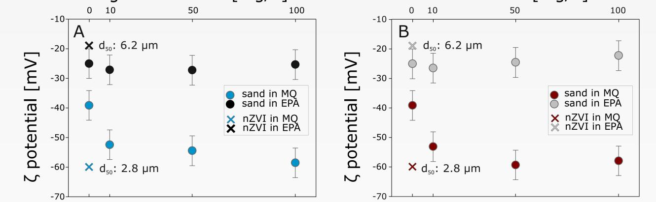
**Zeta (\zeta) potential of nZVI** (calculated from the electrophoretic mobility) and **of sand** (calculated from the streaming potential) measured in a sand column modified with **lignin** sulfonate (A) and humic acid (B) solutions in MQ and in EPA water. Note that the  $\zeta$ potential of both sand and nZVI is significantly lower in MQ than in EPA water and that the <u>nZVI aggregates are larger in EPA</u> than in MQ water.
