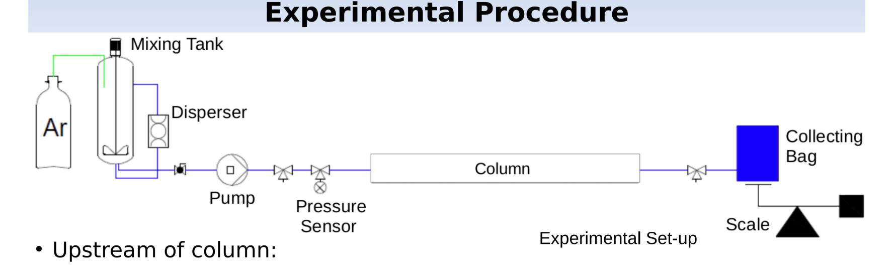
Argon as inert gas, disperser and stirrer to **avoid sedimentation and agglomeration**, peristaltic pumps, pressure sensor for monitoring the pressure, sampling valve for inflow sample.
