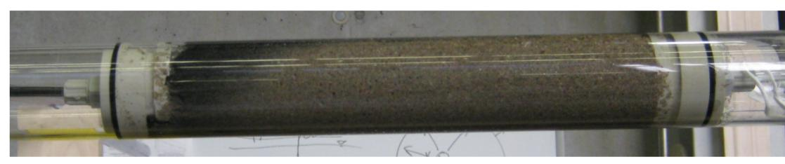
Injection of CI slurry into a column
