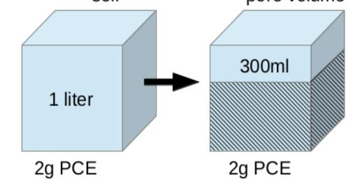
10m<sup>3</sup> of soil, with 2g PCE per liter of soil, or rather 2g PCE per 300ml of pore volume (PV), then 10g ZVI per 300ml PV are required for the remediation.
