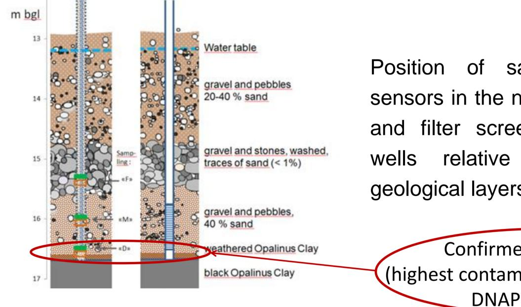
sampling points/iron sensors in the new monitoring wells and filter screen of the injection relative to different the geological layers of the aquifer.
