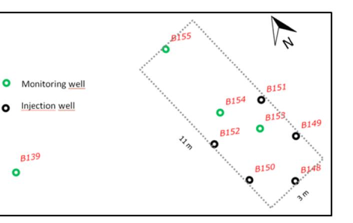
A pump-and-treat system has been in operation for 12 years, but the efficiency of this installation is decreasing, thus there is an interest in alternative technologies for groundwater remediation. Injection of nanoscale zero-valent iron (nZVI) is an innovative technology, which could have the potential to expedite the remediation. The flake shaped, milled nanoiron FerMEG12 was selected for this field-scale pilot test because of its special physical-chemical properties.
