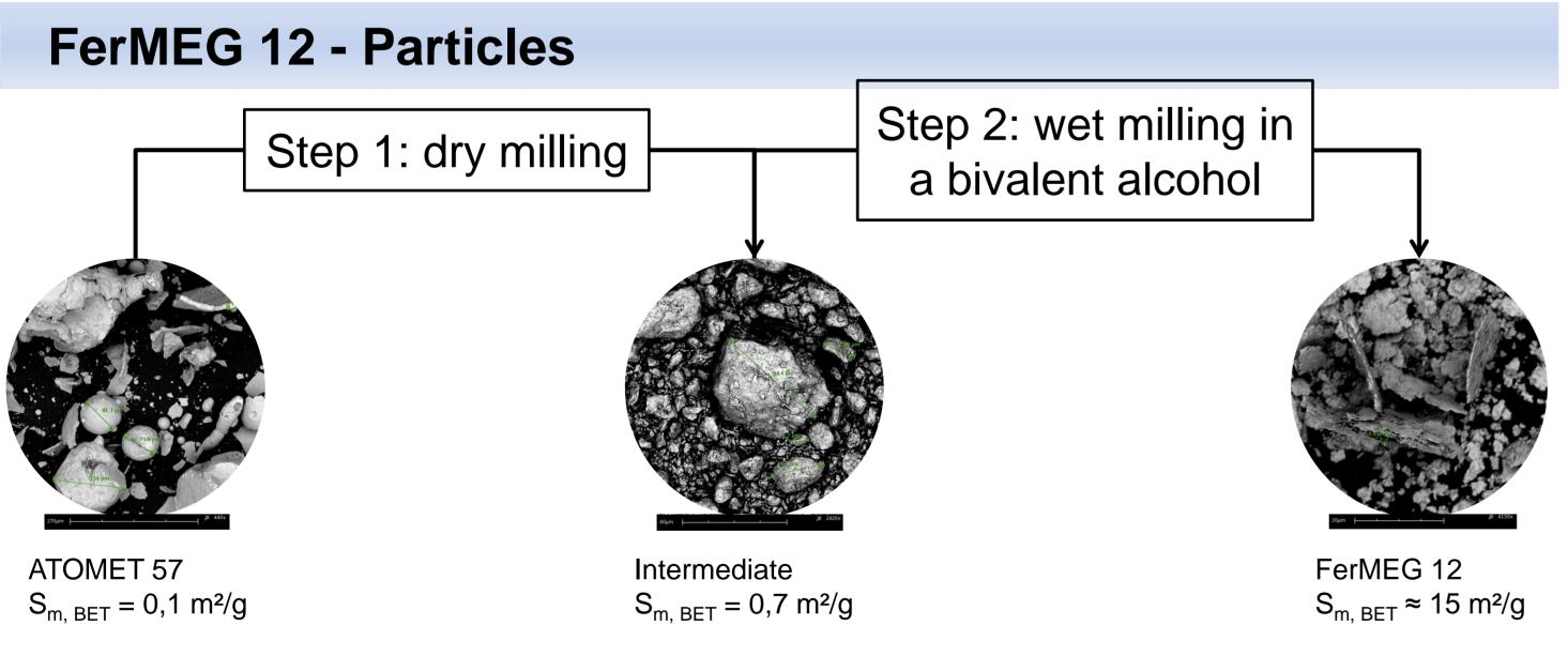
The particles are produced in a two-stage top-down process. Dry grinding to get particles < 40  $\mu$ m, followed by grinding in a bivalent between 5 and 7 atm.
