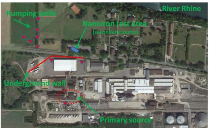
The Zurzach site is located in the Rhine valley northern in Switzerland. The main groundcontaminants are PCE, water TCE Hexachloroethane and (HCA) which were manufactured at this site until 1976.
