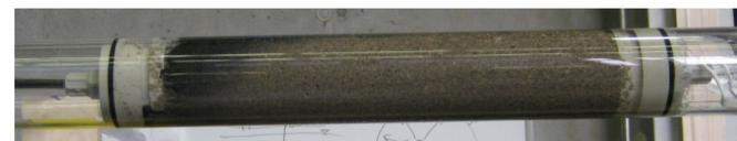
Injection of CI slurry into a column
