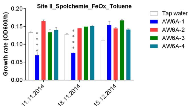
Figure 1, showing reduced toxicity of groundwater close to an injection well (monitoring well AW6A-1) at the polluted site Spolchemie II (assessed as growth rate of the bacterium *Clostridium perfringens* by the Technical University of Liberec), within three weeks after iron oxide (FeOx) nanoparticles.
