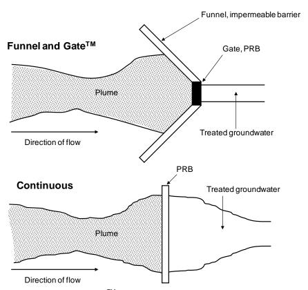
Figure 4: Funnel and Gate<sup>™</sup> and Continuous PRB Configurations (from Nathanail et al. 2007)
