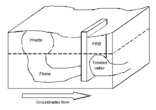
Figure 3: Typical PRB Configuration (from Nathanail et al. 2007)
