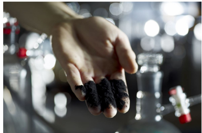
Figure 1. Air-stable Carbo-Iron® contains iron NPs sorbed to activated carbon (Photo: A. Kuenzelmann, UFZ).
