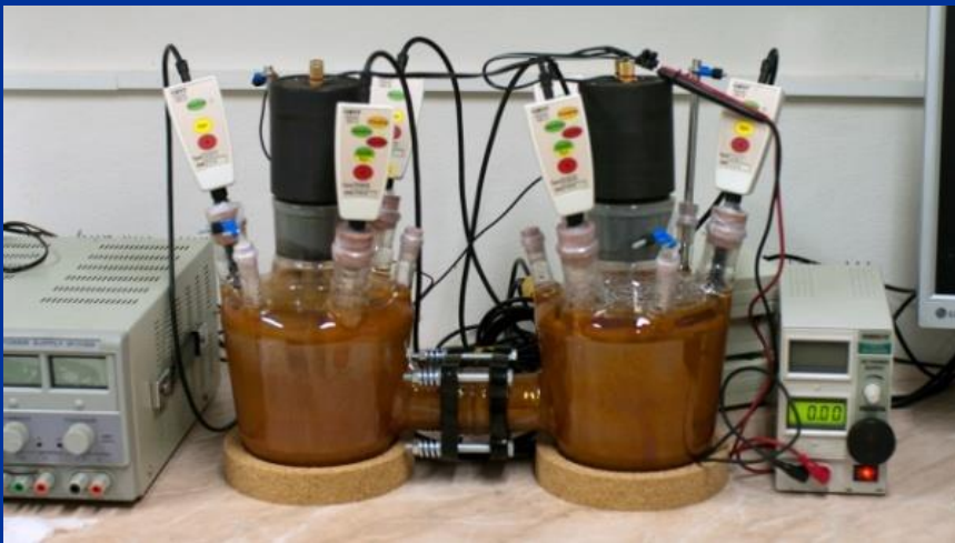
Separated electrodes space (ion membrane)
