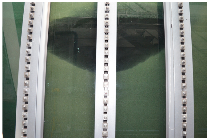
Figure 4. Spreading of Carbo-Iron® suspension in the large scale flume (LSF) experiment © VEGAS/USTUTT, University of Stuttgart, Germany.
