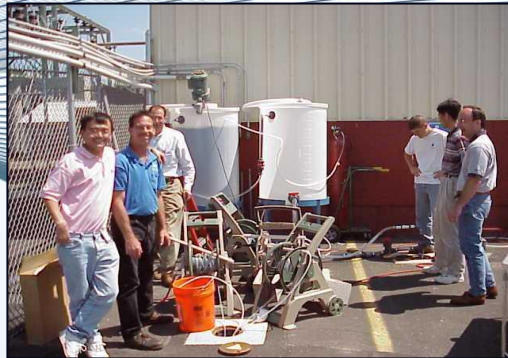
Pre-injection Batch Mixing of nZVI Slurry
