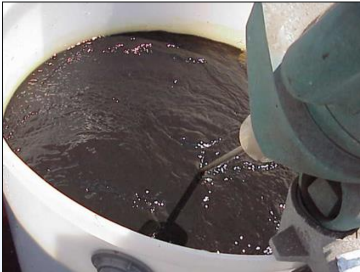
Pre-injection Batch Mixing of nZVI Slurry (Photo: Dan Elliott) First field-scale demonstration, Trenton, NJ, 2000
