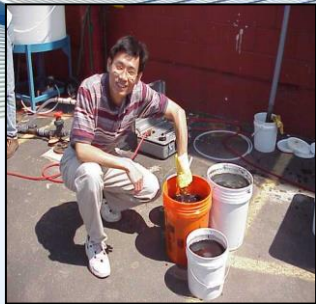
Pre-injection Batch Mixing of nZVI Slurry
