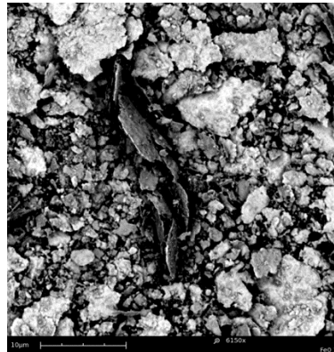
SEM pictures: starting product ATOMET57, pre-milling product, FerMEG final nZVI
