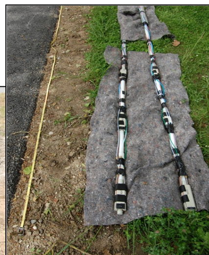
(Right) Monitoring arrays for in situ susceptibility measurement ready for installation on pilot site (© VEGAS/University of Stuttgart, Germany)
