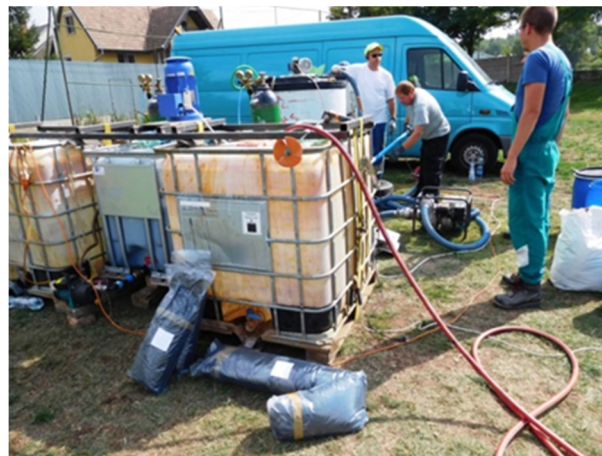
Figure 5. Equipment to prepare Carbo-Iron ® suspension (prior to mixing).
