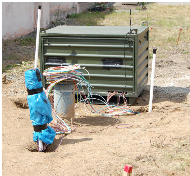
Figure 6. Heads of monitoring arrays for in situ susceptibility measurement (on Spolchemie I pilot site) connected to measuring hardware in protective box © VEGAS/USTUTT, University of Stuttgart, Germany.
