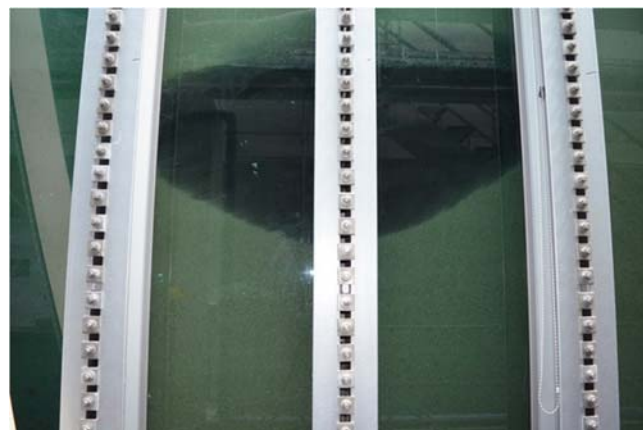
Photo 2: Spreading of Carbo-Iron® suspension in the large scale flume experiment. Source: VEGAS/USTUTT, University of Stuttgart.
